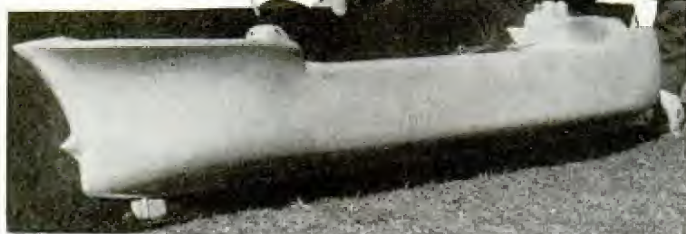
Model of wooden ship designed to ride low and carry warplanes
